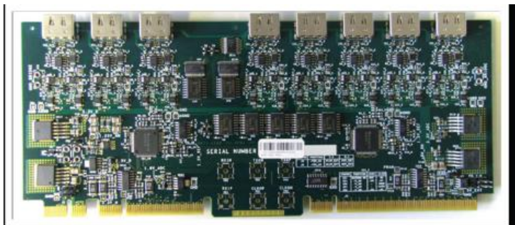
II - The CERN ADC add-in card. PMT readout
