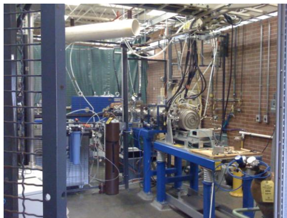
Figure 3. HRIBF Ion Source Test Facility - (ISTF-2) available to test ion sources for on-line generation of Radioactive Ion Beams (RIBs). The ISTF-2 consist of a HV platform, ion source, motor generator, cooling system, Einzel lenses, 90 deg. Dipole magnet for mass separation, Faraday cups for measuring beam intensities, and an emittance measurement apparatus. The room measures 15 m x 10 m x 3.3 m.
