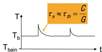
Energy deposition  $E_0$  in the absorber :  $\Delta T = E_0/C$
