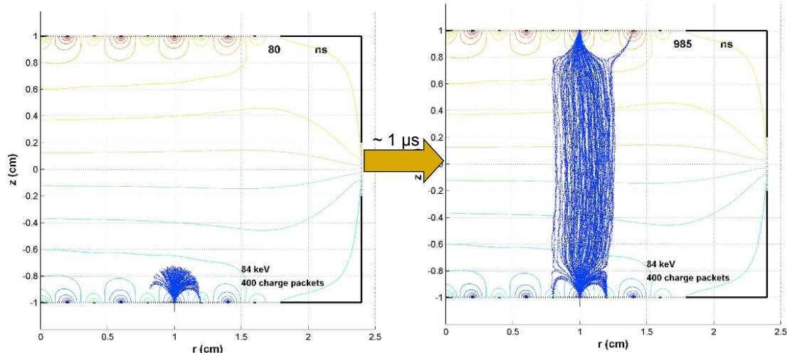
Simulation : interaction under a collecting electrode
