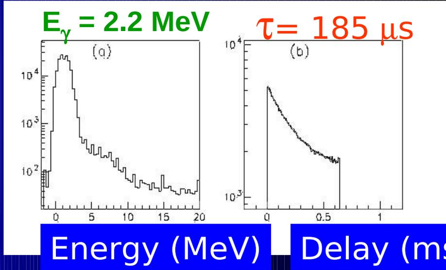
Neutron capture efficiency = 60% (from  $^{252}\text{Cf}$  measurement)
