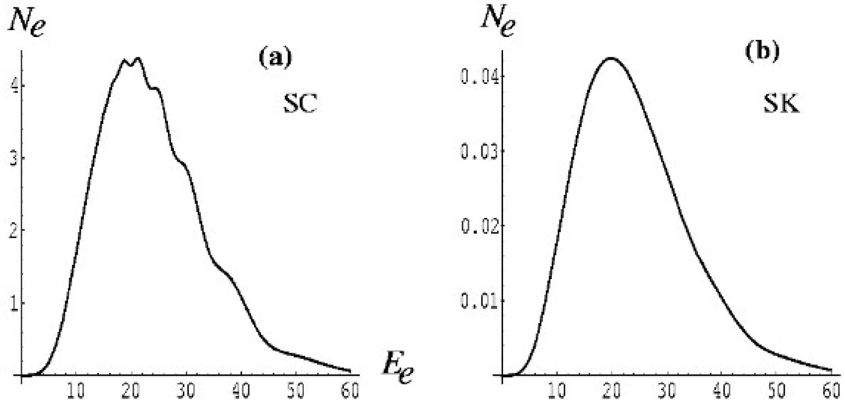
The modulation can be seen by one single detector only if the energy resolution is good enough  $\rightarrow$  **scintillator detectors**
