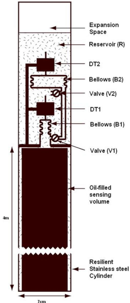
Constructed by Sacks et al. (1971) and widely deployed, consist of a stainless-steel cylinder cemented into a borehole, with a sensing volume filled with silicone oil.
