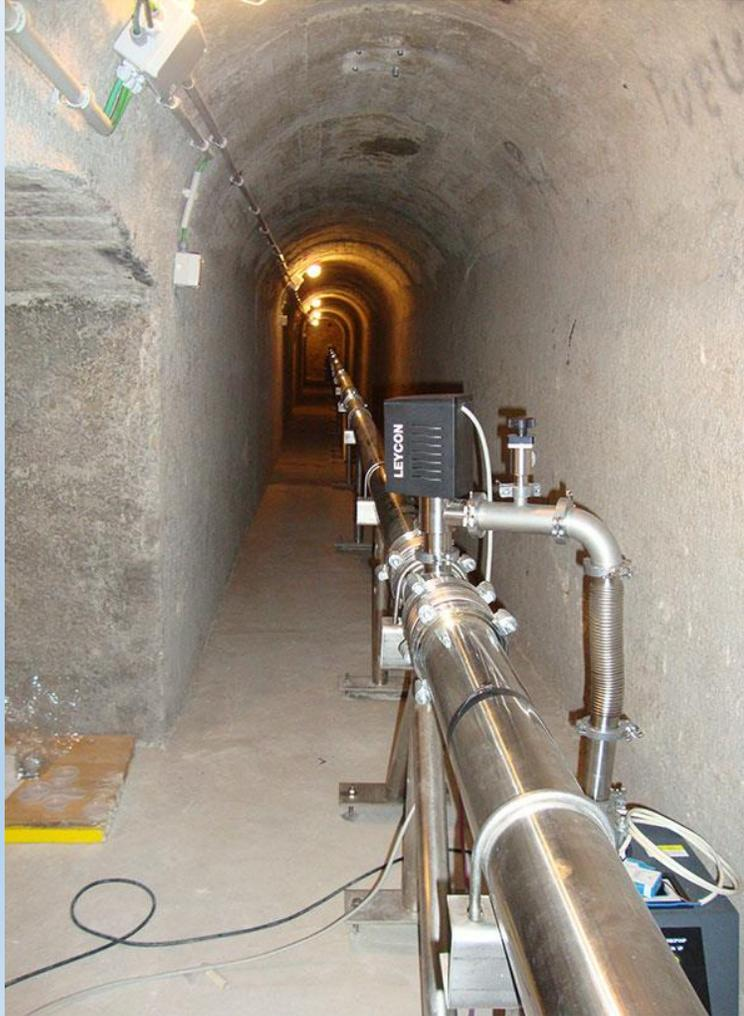
Laser strainmeters (80 m long) installed at the south tunnel of the **Pizzi Deneri Observatory** (Etna volcano - Italy). Part of the pipeline in the lower left.
