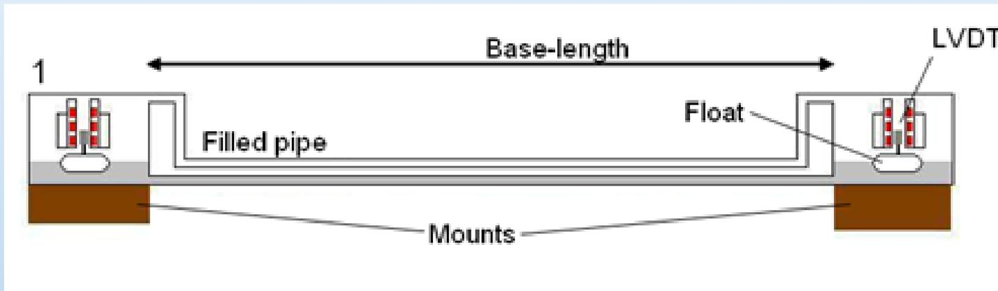
The current water tiltmeters design uses float sensors whose vertical positions are monitored by Linear Variable Differential Transformers (LVDT) with a range of  $\pm 6$  mm and a nominal resolution of  $0.1 \mu\text{m}$ .
