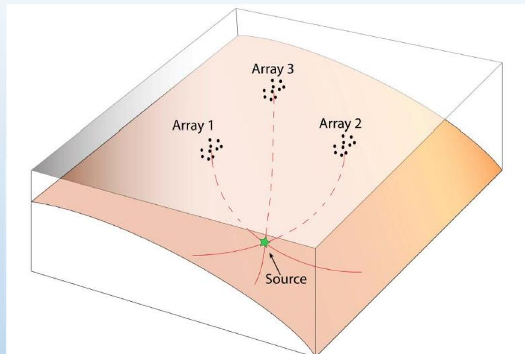
Schematic diagram showing basic idea behind multibeam-backprojection (MBBP) algorithm
