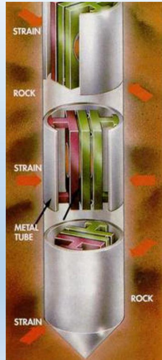
First installed in 1977, this borehole tensor strainmeter is built by GTSM Technologies in Queensland, Australia. The US Plate Boundary Observatory (EarthScope, UNAVCO) installed 74 GTSM during 2005-2008
